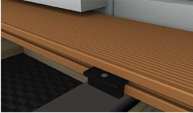
**4** In the groove across the edge of the Bamboo Board, position Fixing Clips and screw into supporting Joists using Screws provided, for every supporting Joist use one Fixing Clip. Our Stainless Steel Wood Screws are recommended as they offer increased durability with less corrosion. **A 6-7mm gap between Decking Boards is created by Fixing Clips.**
