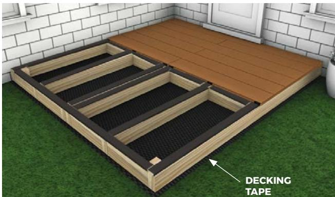
**5** Slide the next Board onto the secured Fixing Clips from the first installed Board, fit a Fixing Clip set to fasten the alternate side of your Board, a single Fixing Clip is to be used per supporting Joist. To fit the rest of the Boards, proceed with a similar method. Make sure the Decking Board ends are fully supported. It is advised to have no cantilever or overhang.
