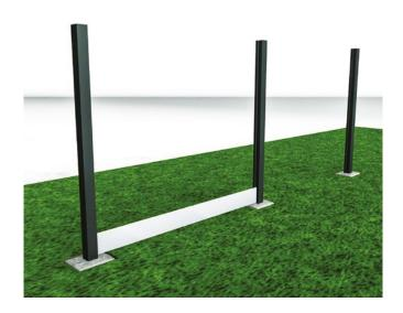
When using the slot between I method, Fence Panels need to be cut into 1.8m lengths. Posts must be 1.8m apart and include an extra 5mm gap each end to allow for expansion of the Panels.
