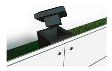
3 Once the desired height has been reached (no more than 2.25m or 10 Panels) simply place the Composite Fence Cap on top of the Post. These are also available in all eight colours to match your Composite Fence. Fence Post Caps simply sit on top of the Post and do not need to be secured.
