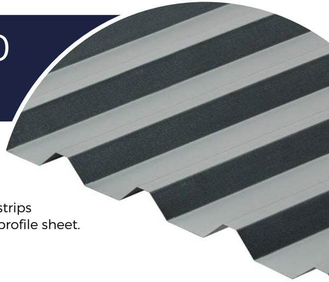
34/1000 trapezoidal box profile roofing sheets are our most popular and strongest profile sheet, with each single skin profile sheet having 7 strong 166mm profiles across its width. Box profile roofing sheets are formed from 1250mm wide steel strips which will give a secure weatherproof lap from profile sheet to profile sheet. Available in 0.5 or 0.7 mm thickness.
