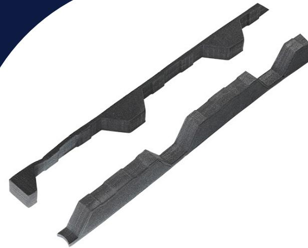
Pairs of polyurethane 32/1000 Box Profile Foam Fillers are used under the Sheeting at the eaves and between the Sheeting and Flashing at the ridges, to close off the Roofing Sheets and stop the elements from affecting your new construction.
