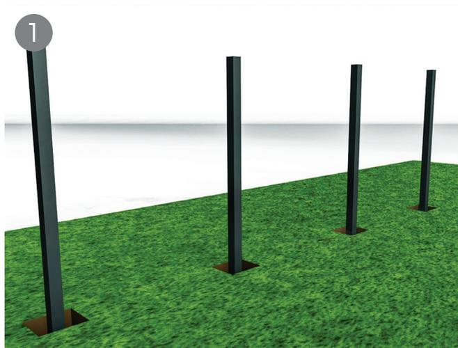
1 Prepare your area by removing any stones, debris or hazardous material. Dig the fence post holes to 25% of the post height. The fence posts must be a maximum of 2m apart to ensure they can support the fence panels.
