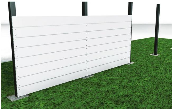
**2** As you start to add more Panels ensure each Panel is 100% level before fixing. Each Fence Panel slots on top of the Panel previously fitted. (Example shows 3.6m Fence Panels with a Fence Post in between).
