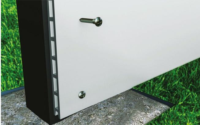
**1** Alternatively, each 3.6m Panel can be secured to the front of the Post, with a supporting Post every 1.8m behind to provide stability. When adding the first Fence Panel, ensure it is 100% level before fixing to Posts. Screw the top and bottom of each Fence Panel to the Fence Posts behind.
