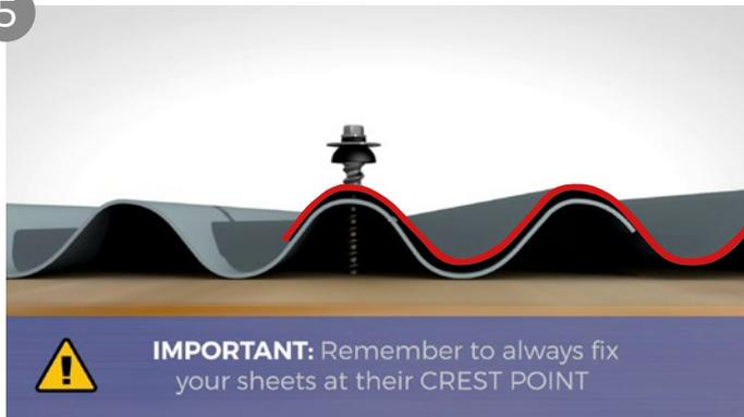
When fixing your corrugated sheeting its imperative they are fixed at the crest point, we recommend using 65mm BAZ screws which are self drilling and self sealing. Please see image above.
