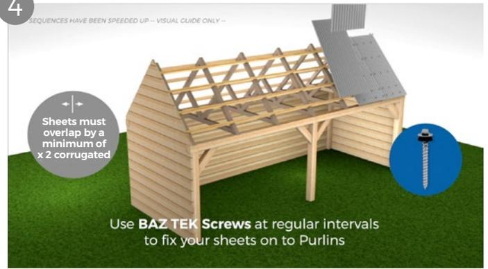
When installing the corrugated sheeting you may wish to lay the sheets on the roof before fixing to ensure the overlap is sufficient. Sheets should be overlapped by a minimum of two corrugations when laid side by side. Colour caps can be used to cover the silver screw head and matched to the roofing sheet colour.
