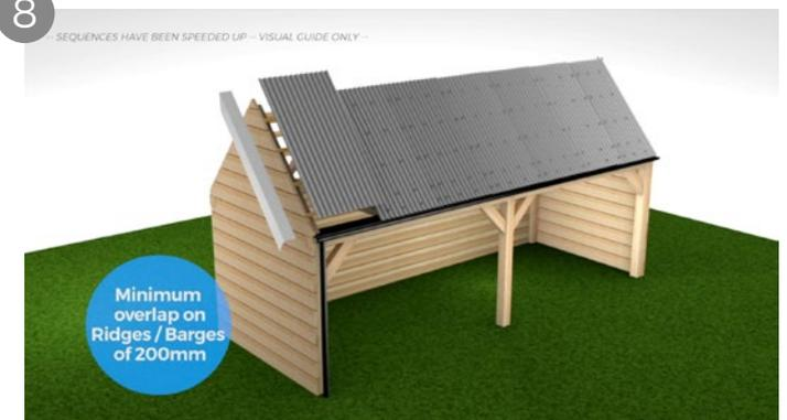
Once you have installed the final sheet you can use Cladco flashings for the sides and apex. Barges are used on the edges to help seal the building and provide an aesthetically pleasing affect. Please note when joining / laying these there is a minimum overlap of 200mm on barges. Sticher screws at 22mm are advised for securing flashings in place.
