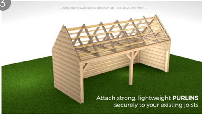
The minimum pitch needed for corrugated sheets is 10 degrees. If in doubt consult an engineer. The purlin spaces on average should be approximately 1.2m apart, however if using 0.5mm for the roof (which is normally used for side sheeting) you would need to reduce purlin spaces to no more than 1m apart. Please note, these are recommended spacings but always seek advice from a structural engineer before installing.
