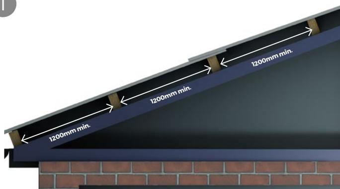
The minimum pitch needed for corrugated sheets is 10 degrees. On a two sheet run its imperative to have a purlin underneath the sheets overlap as shown in the image above. This can vary dependent on your roof construction and degree of pitch. The purlin spaces should be no more than 1.2m apart, however always consult a professional prior to completing any work.
