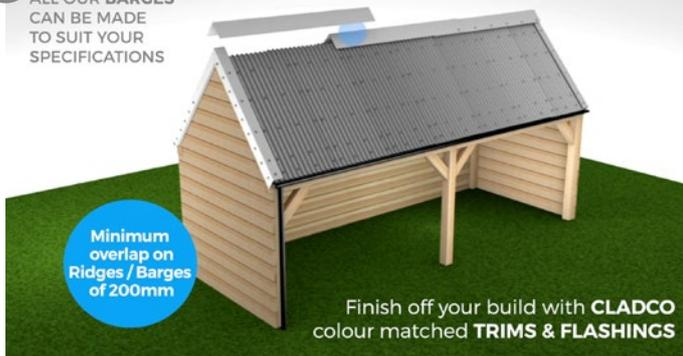
Ridge Flashings are used for the ridge on an Apex roof, where as for a single slope roof you may need to use a custom flashing. To fit the ridge use stitcher screws fix into the flashing and onto the rib/raised profile of the sheets. Lay ridge caps from the opposite end of the roof to the direction of prevailing winds. Each ridge should be overlapped by a minimum of 200mm.
