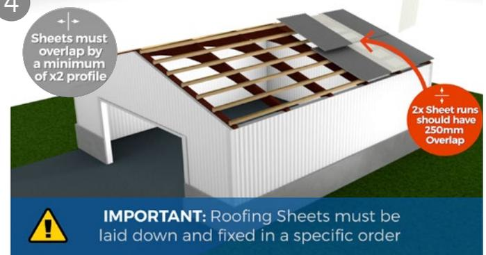
Sheets must be overlapped by a minimum of 250mm where the two sheets meet. Roof lights can be installed between the sheets but must have sheets either side for support. Sheets should overlap side by side by at least two corrugations.
