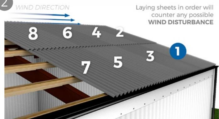
For a two sheet run, sheets should be laid in a particular order to the prevailing wind. Start at the eaves and in the corner away from the direction of the prevailing wind (this will help to prevent side laps facing into the wind and water ingress). If the first sheet is not laid perpendicular to the eaves and ridge, adjustments will have to be regularly made when laying other sheets and a 'saw tooth' effect at the eaves will be seen.
