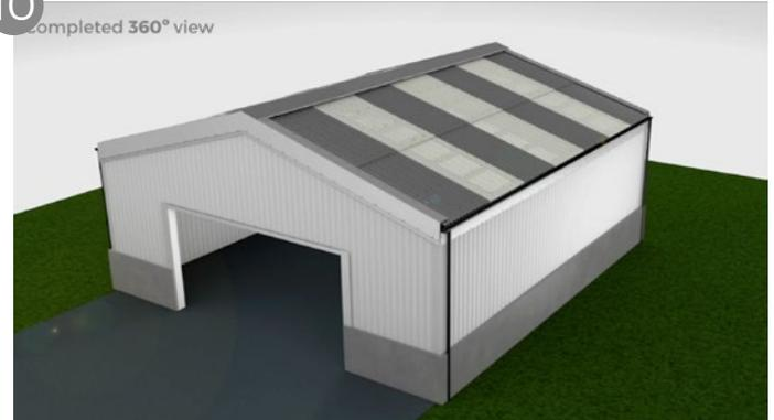
Finish your project by installing the ridge flashing along the centre where two sheets meet. You can then install guttering or fascia as required.
