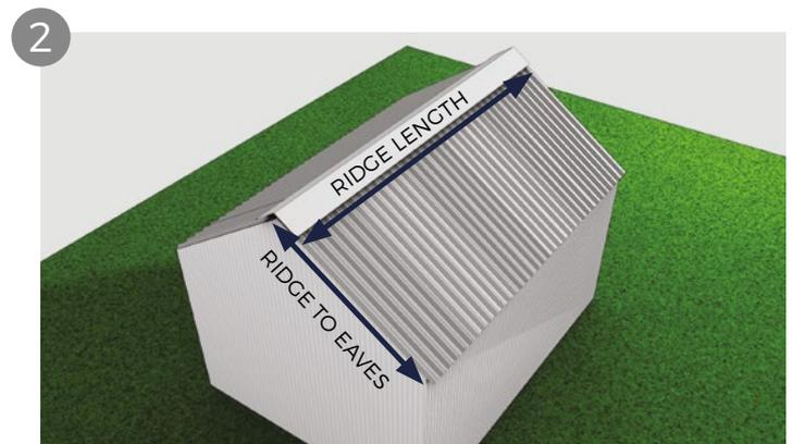
Apex roofs are separated by a central ridge. As per the diagram we require the length of sheet from ridge to eaves and the ridge length to calculate your requirements. You will need to measure both sides of the roof as the building/roof can vary in size from side to side. If the apex is uneven ridge to eaves will need to be taken on both sides.
