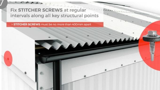
Stitcher screws are recommended to secure flashings. Screws should be no more than 400mm apart when securing the flashing. Colour caps can be used to conceal the top of the screw head.
