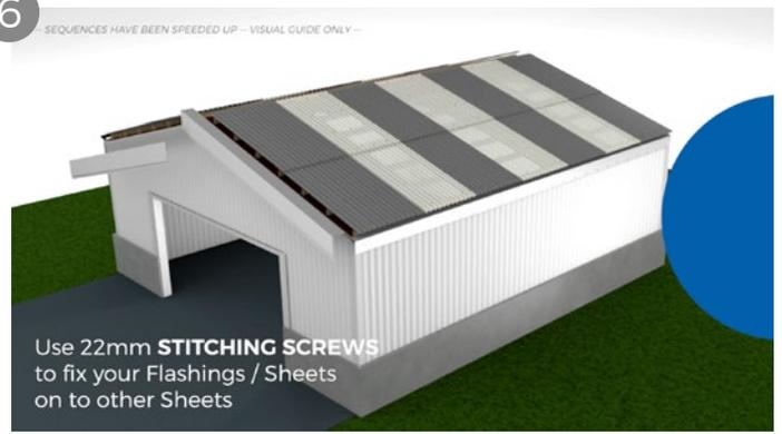
Barge flashings can be used to seal and finish off the ends of your roofing project. Flashings can ensure the building is watertight and prevent birds and water from entering the building. It is good practice to use mastic lapping tape and stitching screws to ensure a robust weather resistant joint on side laps.
