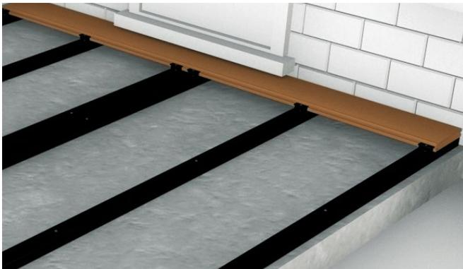
**6** Each Board should be held into place with a Fixing Clip where two Board ends meet. Allow 2mm of spacing between butt joints.
