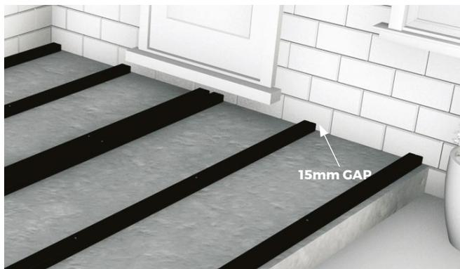
**2** Before your first Decking Board is placed, a Starter Clip must be fixed on to the Composite Joists end. Starter Clips need to be placed at every Joist end where your Bamboo Boards will lay. A slight gap should be left between the Joist end and any walls.
