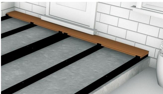
**4** Fixing Clips are then slotted into the Boards groove on the side and screwed into your supporting Joists with Screws provided, an individual Fixing Clip is used per Joist. We suggest opting for our Stainless Steel Wood Screws due to their durability and reduced chance of corrosion. Between your Bamboo Decking Boards, Fixing Clips will give a **6-7mm break between Boards**.
