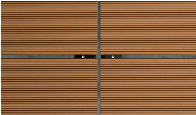
**6** Where two Bamboo Board ends meet (butt joints), each Board must be 2mm apart from each other and Fixing Clips must hold each Board into place at the meeting point.
