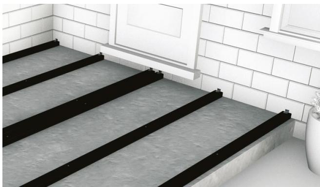
**3** Our Bamboo Boards are fastened easily to supporting substructure Joists, our Fixing Clips and Stainless Steel Screws allow for simple installation. From the outer sides of your structure, lay your first Bamboo Board and, with a row of Starter Clips, fix on each Joist that it crosses.
