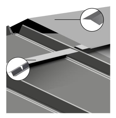
O Slide the Ridge Flashing over the O Z Bars on both sides to fit into place. Secure the Flashing by clamping the edges using hand seaming pliers to fix the Flashing into place. For Mono Ridge Flashings, pull the Flashing over the Backer Plates and Z Bars and clamp into place.
