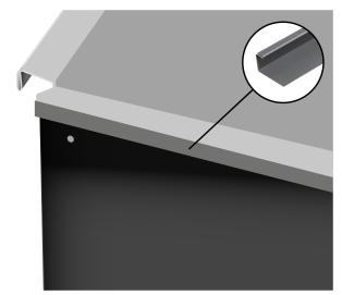
Position and secure the Sheet over the seam using a rubber mallet to tap into place. Using Ring Nails, secure the left side of the last Sheet down the edges of the corner (one nail every 200mm).
