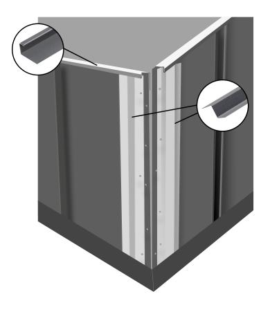
Measure and cut Z Bars to fit at the corner of a wall on either side. Install one Z Bar 90mm from the exterior edge. To better gauge its position, place a Corner Flashing section over the Bars and mark where the Z Bar will go on the adjoining wall.
