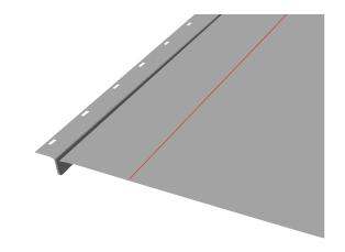
Repeat the previous step until you reach the final Sheet. Measure the width of the final Sheet and add 25mm for the Verge upstand. Cut off the fixing holes and fold the 25mm upstand along the left-hand side and top edge using hemming tools. The max width of this Sheet will be 470mm.
