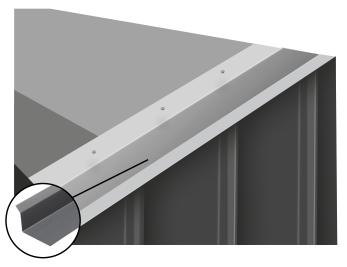
If you are installing a mono-pitched roof, start by measuring and fixing Mono Ridge Backer Plates along the top edge of the roof using Annular Ring Nails. If you are installing a dual-pitched roof, move on to the next step.
