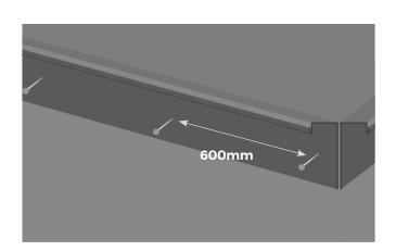
To secure a J-Rail Flashing, fix Ring Nails through the 60mm flat section. Five nails per length of Flashing should be used. Apply butyl tape or silicone sealant behind the J-Rail Flashings before securing them into place.
