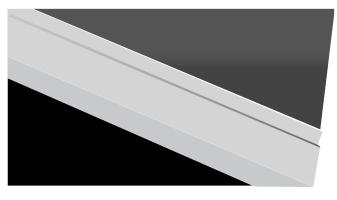
Tap the final Sheet at the base to nudge it into position over the Eaves Flashing and tap over the seam to secure it in place. Ensure Sheets are fully clipped together. The left-hand edge should align with the Verge Backer Plate.
