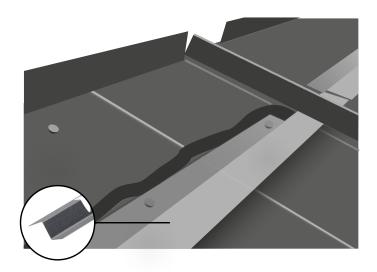
To install the Ridge Flashing, align the Z Bars (Notched) along the top of your roof. To help do this, temporarily place a Ridge Flashing or Mono Ridge piece over the apex and mark the position of the Z Bars. Use a string line and chalk mark to place Z Bars.
