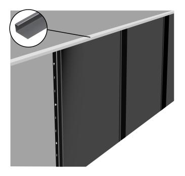
Secure the Sheet in place using Ring Nails every 3-4 fixing holes (200mm). Continue securing the rest of the Cladding Sheets following the previous step until you get to the last Sheet. Measure the width of the final Sheet and cut it to size along the fixings side of the Sheet to complete the final run of Cladding along the wall.
