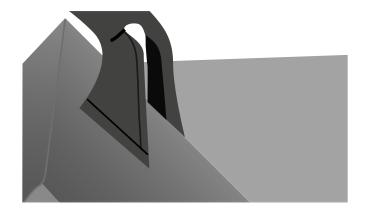
5 Using seaming pliers, clamp the bottom and top edges of the Verge Flashing around the Verge Backer Plate and upstand to create a tight seal. Finish each side of the roof with a Verge Flashing piece.
