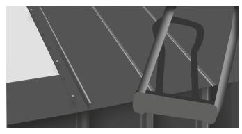
Working from right to left, measure the width of the first Standing Seam Sheet and include 25mm for the verge upstand. The maximum width of the first sheet will be 445mm after cutting off the seam.
