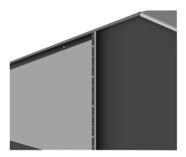
Continue to install Sheets to all walls and at gable ends, adjusting the angle of the cut edge according to the roof's pitch. Sheets can be centralised with the apex of the roof and fixed in place using Ring Nails every 3-4 fixing holes (every 200mm).
