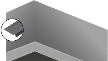
Measure and cut the Verge Flashing to length and install over the 25mm upstand and Backer Plate. For apex roofs, cut at an angle to sit flush with the adjoining Verge Flashing at the apex.
