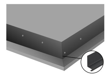
When using Ring Nails, fix centrally in TOP TIP the fixing holes to allow for expansion and contraction in both directions.
