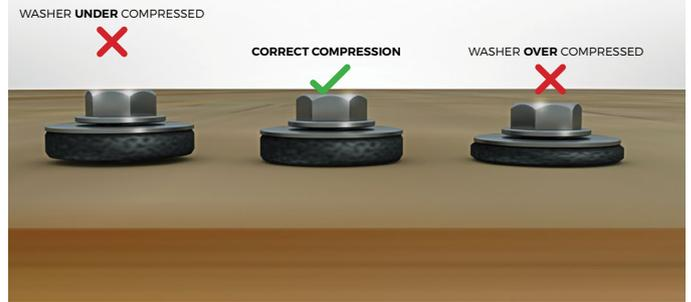
**TOP TIP** Do not over-tighten or under-tighten your screws as this can affect the performance of the washer and prevent it from sealing correctly. See diagram above.
