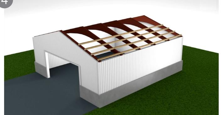
The minimum pitch needed for tile sheets is 12 degrees. On a two sheet run its imperative to have a purlin underneath the sheets overlap as shown in the image above. This can vary dependant on your roof construction and degree of pitch. The purlin spaces should be no more than 600mm apart, however always consult a professional prior to completing any work.
