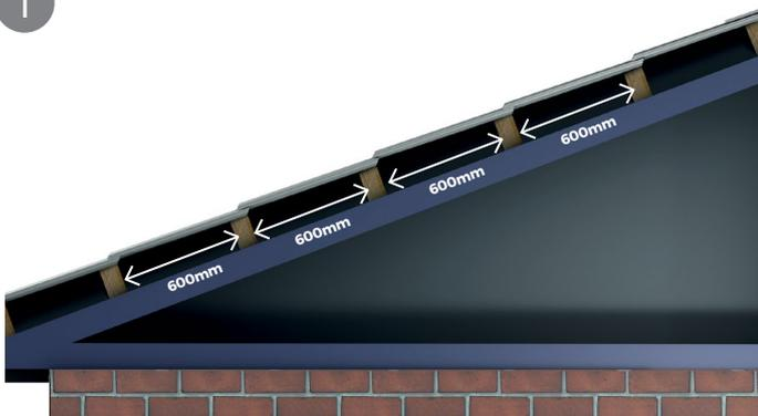
Purlin spaces for tile sheets need to be 600mm apart. These need to be in the correct place to be able to fix correctly at the top end of every second tile as shown.
