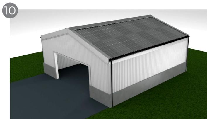
Finish your project by installing the ridge flashing along the centre where two sheets meet. You can then install guttering or fascia as required.
