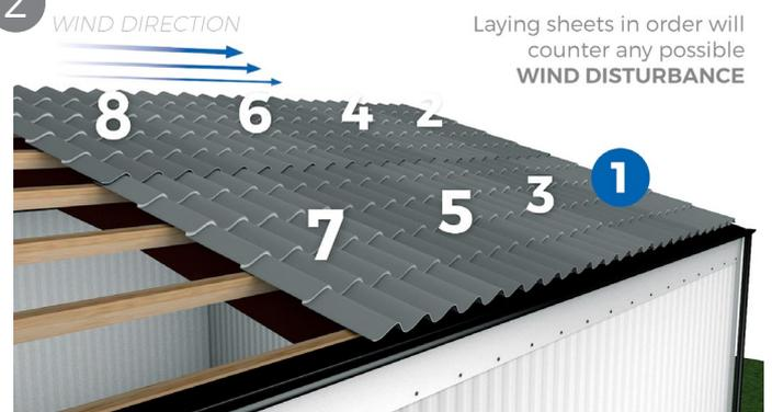
For a two sheet run, sheets should be laid in a particular order to the prevailing wind. Start at the eaves and in the corner away from the direction of the prevailing wind (this will help to prevent side laps facing into the wind and water ingress). If the first sheet is not laid perpendicular to the eaves and ridge, adjustments will have to be regularly made when laying other sheets and a 'saw tooth' effect at the eaves will be seen.
