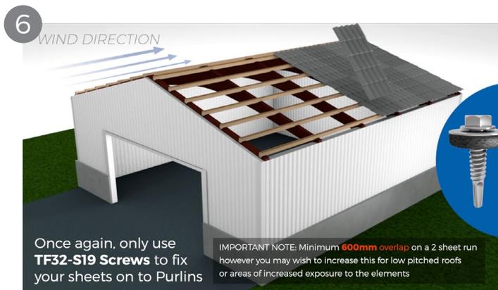
Sheets should be overlapped by the next sheet in the run by at least one tile profile ('side laps'). Adjacent runs of sheets should overlap each other by at least 600mm. Please note, we can only supply maximum length of 5 metres. If you require a longer length, its recommended to do a two sheet run.
