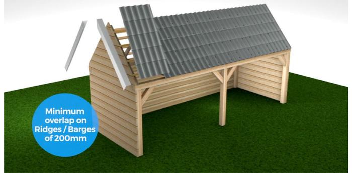
Once you have installed the final sheet you can use Cladco flashings for the sides and apex. Barges are used on the egdes to help seal the building and provide an aesthetically pleasing affect. Please note when joining / laying these there is a minimum overlap of 200mm on barges. Stitcher screws at 22mm are advised for securing flashings in place.
