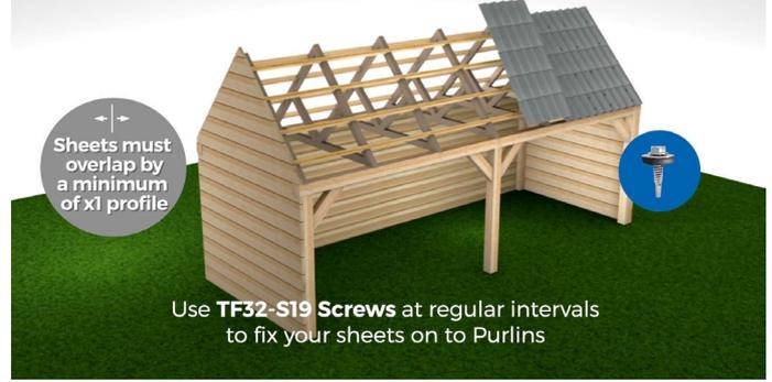
When installing the box profile sheeting you may wish to lay the sheets on the roof before fixing to ensure the overlap is sufficient. Sheets should be overlapped by a minimum of one tile profile when laid side by side.
