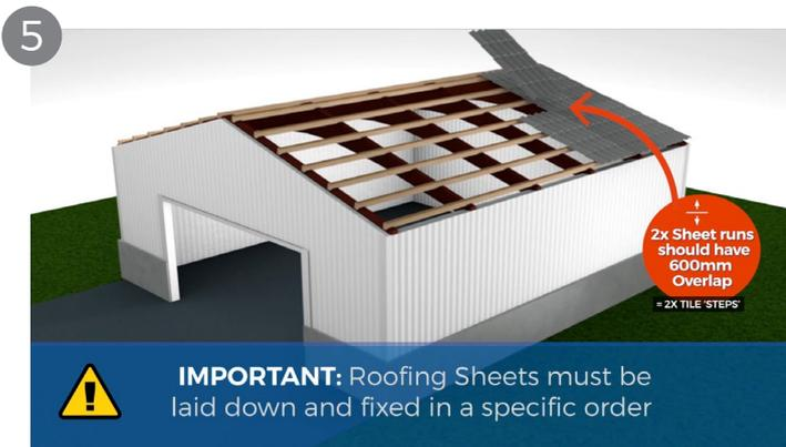
Sheets must be overlapped by a minimum of 600mm where the two sheets meet. Sheets should overlap side by side by at least one tile profile.
