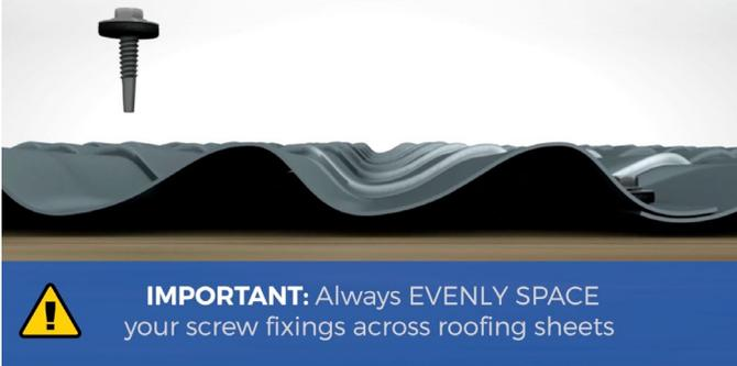
When fixing your tile sheeting its imperative they are fixed at the valley, we recommend using TF32-S19 screws which are self drilling and self sealing. Please see image above.
