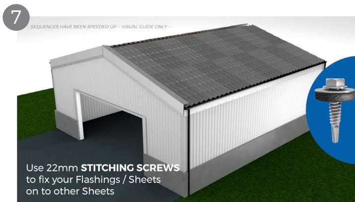
Barge flashings can be used to seal and finish off the ends of your roofing project. Flashings can ensure the building is watertight and prevent birds and water from entering the building. It is good practice to use silicone sealant/adhesive and stitcher screws to ensure a robust weather resistant join on side laps.
