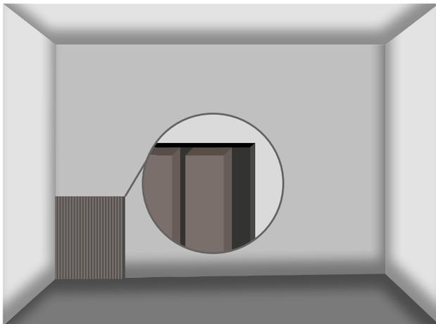
Begin installing onto your wall from left to right. Place your first Slatted Panel up to the wall, ensuring the felt lip is on the right and the wood-veneered slat is flush to the edge of the wall.
