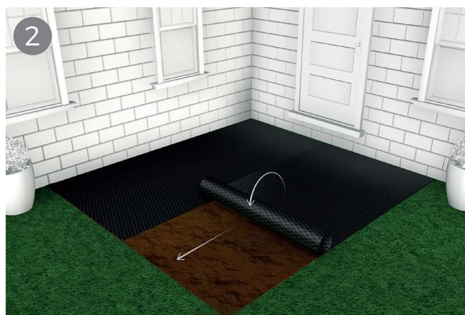
Step 2, Remove the turf until the ground is completely even. Cover the area of your site with a layer of weed control fabric to prevent any weed regrowth coming up under your decking. You may need to cut the weed mat to fit. You may want to pin your weed mat down at this stage.
