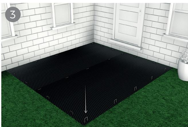
Step 3, Lay your Cladco Weed Mat on top of the prepared soil, if you need to overlap ensure you do this with enough coverage for weeds not to penetrate through. Cover the weed mat with your desired coverage such as chippings, bark or stones so none of the weed mat material is exposed.
