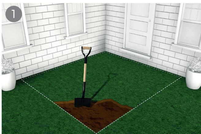
Step 1, Clear away any plants, weeds, rocks, or other material that might be obstructing your site. Cut away the turf or the lawn by using an edger to cut the area and then a shovel to remove it. Make sure the ground is level.
