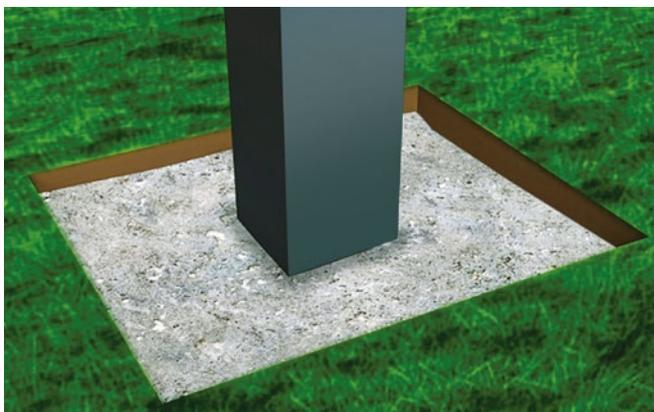
**3** Make sure every Fence Post is 100% level before using postcrete. Fence Posts must have at least 25% of their height concreted into place.
