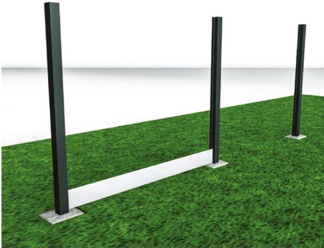
**1** When using the slot between method, Fence Panels need to be cut into 1.8m lengths. Posts must be 1.8m apart and include an extra 5mm gap each end to allow for expansion of the Panels.
