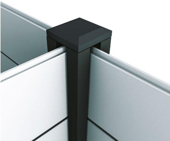
**3** Finish your Fence Post with a Fence Post Cap. Fencing Panels can be finished with Cladco Fencing Rails, manufactured from hard-wearing steel. Rails can be cut down to size using Straight Cut Tin Snips and slotted onto the top of the Panels for neat edge.
