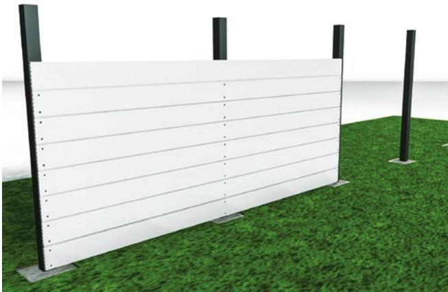
**2** As you start to add more Panels ensure each Panel is 100% level before fixing. Each Fence Panel slots on top of the Panel previously fitted. (Example shows 3.6m Fence Panels with Fence Post in between).
