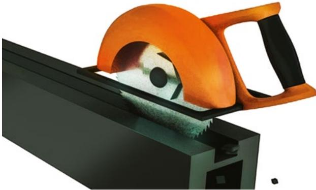
**1** If using the slot between method, cut up to four channels per Post. Please ensure you leave an adequate expansion gap when using the slot in method to allow for natural expansion of the Panels.
