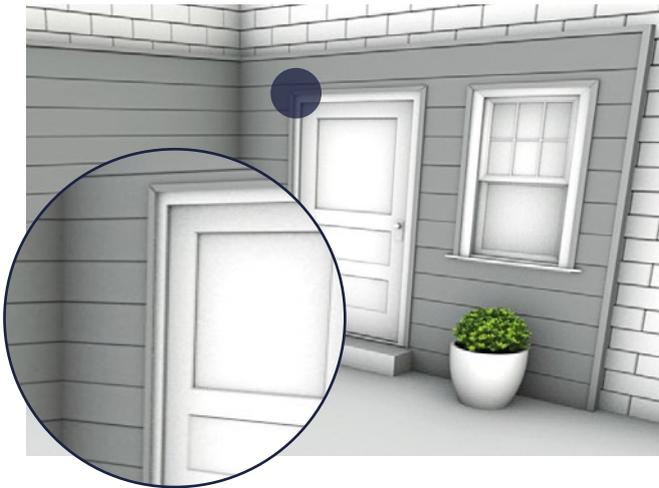
Installing Corner Trims is the last phase of the project. Install Composite Wall Cladding as above right up to any windows or doors.
