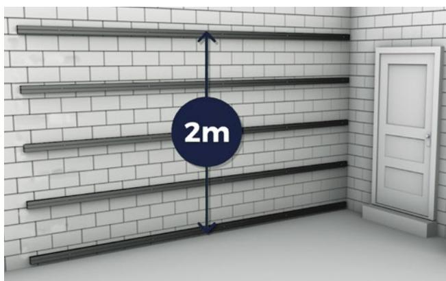
**3** Battens should be attached to the surface at a maximum distance of 500mm apart. The Battens will need to run the entire length of the area being clad, adding in additional Battens at any point where you will need to join two Cladding Boards end to end. Remember to install your Battens at a 90 degree angle to the way that you want your Wall Cladding Boards to run. It is important that the surface below the Battens is flat and stable.
