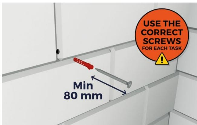
**2** You will need to pre-drill the Battens and the surface below using a 6mm drill bit. Cladco Composite Battens are 30mm high and you will need to secure them at least 50mm into the surface below. You will need to choose fixings suitable for the surface you are fixing into. Screws should be 5-6mm diameter and at least 80mm long\*.
