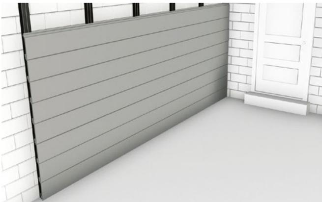
**8** Continue to fit the Cladding Boards in this manner until you have completely covered the area you want. It is possible to fit your Boards side by side by simply butting the two ends up together and allowing for a temperature expansion gap (refer to page 4). You must install more Battens if you wish to do this, as each Board will need to be supported on a Batten where it meets the next Board.
