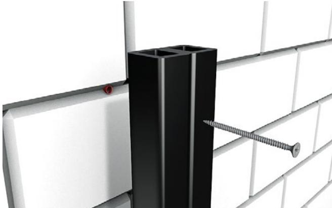
**1** You will need to pre-drill the Battens and the surface below using a 6mm drill bit. The Battens are 30mm high and you will need to secure them at least 50mm into the surface below. You will need to choose fixings suitable for the surface you are fixing into. Screws should be 5-6mm diameter and at least 80mm long\*.
