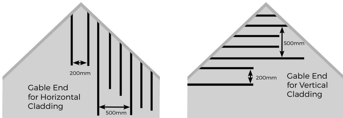
If your home has a gable end, Battens must be spaced up to 500mm apart with additional, shorter supporting Battens installed every 200mm, going up and down the apex (the triangular shape of your gable end). This ensures that the Composite Boards are fully supported across the entire build.
