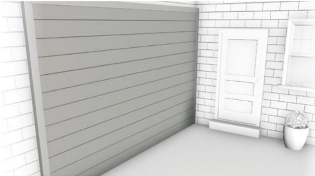
Whether you have installed Composite Wall Cladding vertically or horizontally, you can use matching Composite Corner Trims to complete the look of your project for a professional touch. Composite Corner Trims can be worked into your installation easily using normal woodworking tools and CTI Adhesive.
