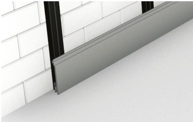
**4** Place the first Wall Cladding Board on to the Starter Strips. Mark and then pre-drill pilot holes through the fixing groove of the Board into the Batten below. Secure the Boards using a screw at least 20mm in length, ensuring that the Board is fastened securely on each Batten that it touches. Secure these fixings by hand, as is important not to over-tighten the screws and risk splitting the Board.
