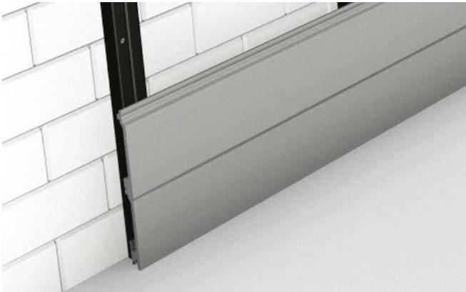
**5** Slot the second Board onto the first and repeat the fixing process ensuring that the second Board is fitted securely in place on each Batten. Repeat this process with each Board until you reach the required height. Ensure that the section between the Battens remains empty to allow air to flow beneath the Boards.
