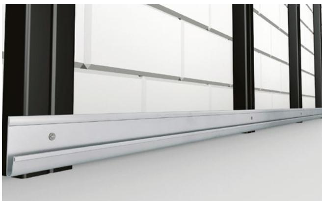
**3** Attach a Starter Strip to the bottom of each Batten, leaving a 10mm ventilation gap at the base of the installation. Ensure no sealant is applied around this area. This will give the first Cladding Board something to sit on. You will need to pre-drill a pilot hole into the Composite Batten and attach the Starter Strip using a screw that is at least 15mm long. Ensure that each Strip is level with the next and that the first Board sits level on the Strips before continuing to the next step.
