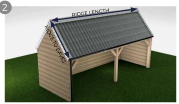
Apex roofs are separated by a central ridge. As per the diagram, we require the length of Sheet from ridge to eaves and the ridge length to calculate your requirements. You will need to measure both sides of the roof as the building/roof can vary in size from side to side. If the apex is uneven, ridge to eaves will need to be measured on both sides.
