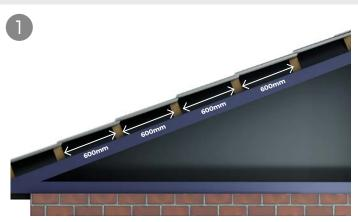
The minimum pitch needed for Tile Form Sheeting is 12 degrees. Purlin spaces should be 600mm apart and Sheets fixed at the top end of every second Tile as shown. If in doubt, consult an engineer.
