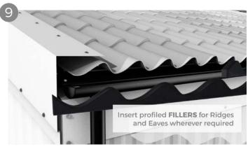
Fillers can help ensure a robust weather-resistant seal to prevent birds and vermin, as well as water, from entering the building. Foam Fillers are designed to go under a Sheet at the eaves and over the Sheet at the ridge. All Foam Fillers should be bonded to the Sheeting with a flexible, waterproof silicone sealant and should be continuous over the entire width of the Sheeting.
