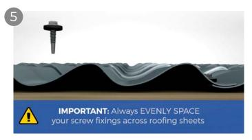
When fixing Tile Form Sheeting, it's imperative they are fixed at the valley. We recommend using TF32-S19 Screws which are self-drilling and self-sealing. Please see image above.
