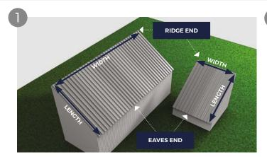
A single slope roof is sometimes referred to as a mono pitch or lean-to roof. When working out your Sheeting requirements, we require the length and width as shown in the diagram for us to be able to help you with a quotation. A width measurement is used to calculate the number of Sheets required. The length measurement is used to calculate the length of Sheets required.
