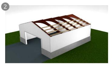
Sheets must be overlapped by a minimum of 600mm where the two Sheets meet. On a two-Sheet run remember to have a purlin under the overlap. These are guides and it depends on your roof's construction and pitch.
