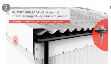
Stitcher Screws are recommended to secure Flashings. Screws should be no more than 400mm apart when securing the Flashing. Cladco Colour Caps can be used to conceal the top of each Screw.
